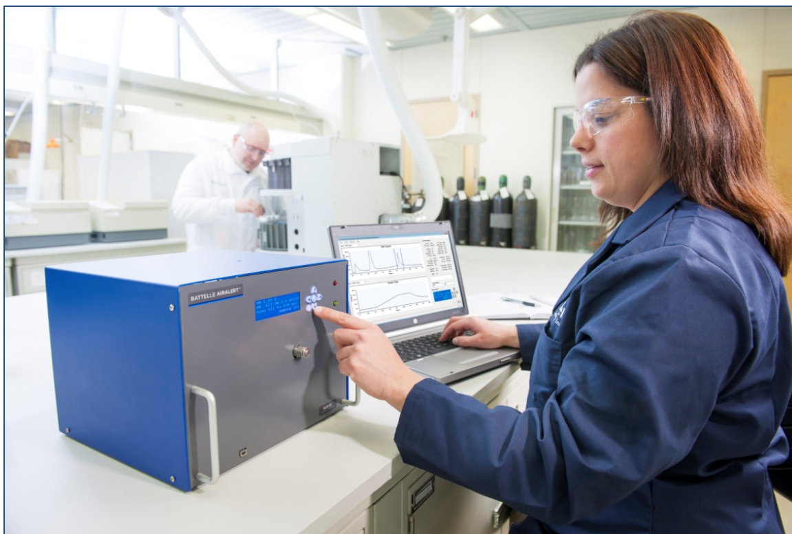
Figure 1. Battelle's AirAlert—an automated air monitoring system.
